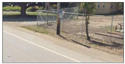
Bus stop lacking sidewalk, a concrete pedestrian waiting area, and an ADA path of travel at 2838 Freedom Boulevard, Watsonville, CA
